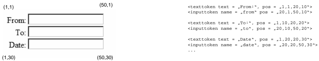
Fig. 6. Simple query interface and result of tokenization
