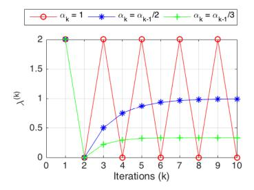
This plot shows that the step length values  $\alpha_k$  play an important role in convergence. When the step lengths are constant, then the  $\lambda^{(k)}$  values oscillate between 0 and 2. If we halve the step length at each iteration, then we converge to the optimal value of  $\lambda = 1$ . On the other hand, if we reduce the step length more aggressively and divide the step length by 3 at each iteration, then  $\lambda^{(k)}$  values converge to a nonoptimal value.
